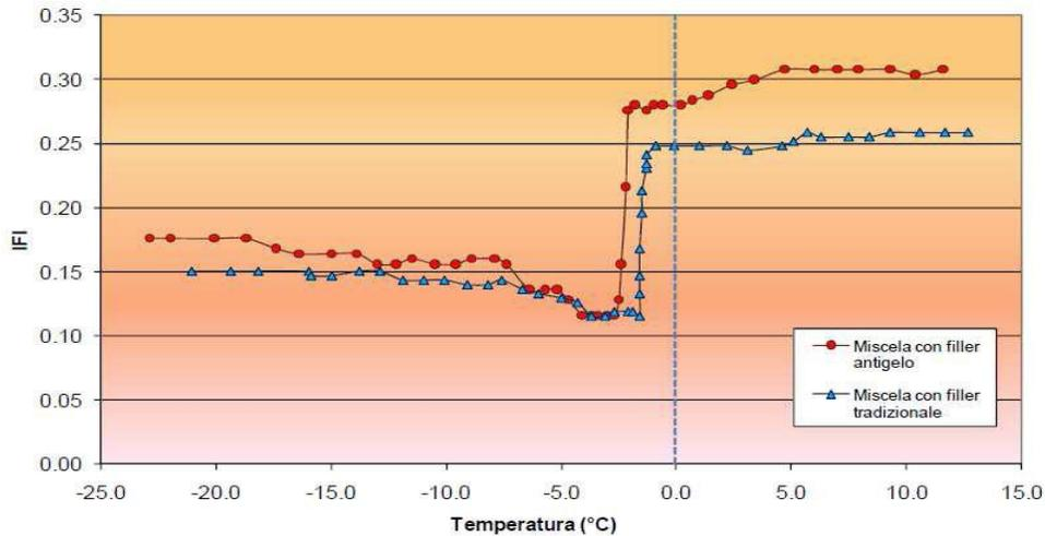
**Graph 2** Trend of the adhesion parameter values IFI-International Friction Index Values determined at the laboratory of the University of Pisa Red: mixture with anti-freeze filler. Blue: mixture with traditional filler
