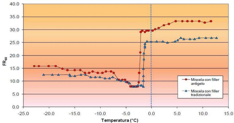
**Graph 3** Trend of the adhesion parameter values measured at the slipping speed of the test pneumatic (FR60 ). Values determined at the laboratory of the University of Pisa Red: mixture with anti-freeze filler. Blue: mixture with traditional filler.
