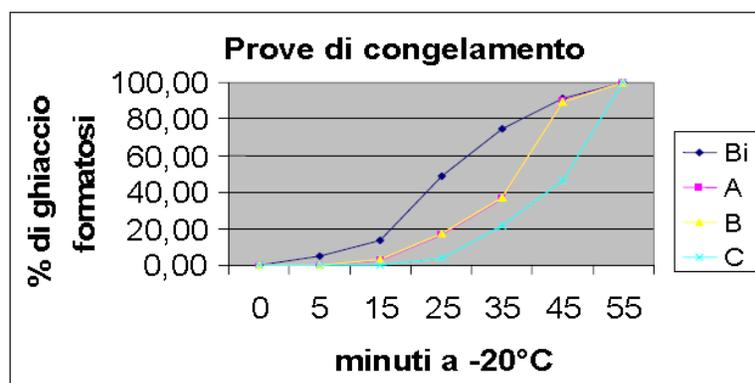
Graph 1 Bi = bitumen itself; A and B = Competitors' anti-freeze and bitumen mixtures at 5%; C = anti-freeze and bitumen mixtures WINTERPAVE-ECO at 5%, calculated on aggregates weight
